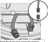
Feed the 9-pin plug connector coming from the bottom of the motor housing through the center hole in the light kit assembly. Connect it to the plug connector found in the switch housing area of the light kit assembly. Make sure to line up the colored markings on the connectors.
