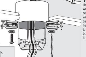
Use wood screws and washers (included) when securing to support structure with approved electrical outlet box. Drill 9/64" pilot holes in support structure to aid in securing ceiling bracket with hardware found in the  $\bigstar$  hardware bag.
