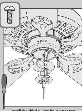
Install the third switch housing screw.
