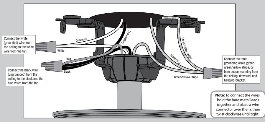
Turn the splices upward and push them carefully back through the hanger bracket into the outlet box. Spread the wires apart, with the grounded wires on one side of the outlet box and the ungrounded wires on the other side of the outlet box.
