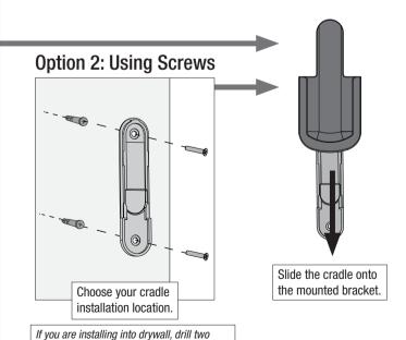
9/64 in width holes using the cradle bracket as a guide. Gently hammer the included drywall anchors into the pre-drilled holes.
