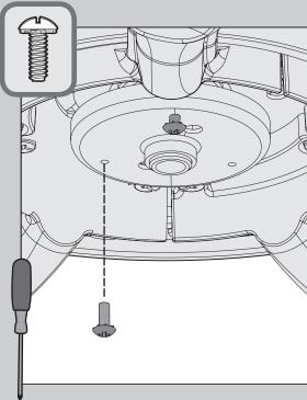
Screw two (2) housing assembly screws from the = hardware bag halfway into the motor housing. It does not matter which two screw holes you choose.
