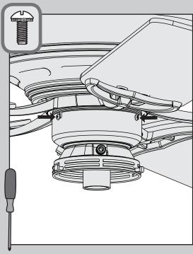
Install the third switch housing screw.
