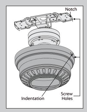
Raise the motor housing up over the motor and ceiling bracket. Turn the motor housing so the screw holes align and the indentation in the housing locks into place with the notch in the ceiling bracket. The motor housing is not secured until the next step is complete.
