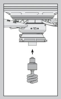
Install a CFL bulb (19-watt maximum).
