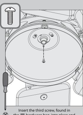
the hardware bag, into place and then tighten all three screws.
