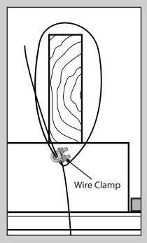
Wrap the braided cable around the support brace once, creating a complete circle. Thread the end of the cable through the bottom of the clamp again so the excess cable hangs out the top. Be sure to remove any slack from the cable.
