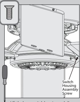
Lift the lower switch housing and align the screw holes with the screw holes in the side of the upper switch housing. Install the three switch housing assembly screws found in the hardware bag.
