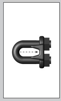
Loosen the two nuts on the wire clamp and slide the clamp open.
