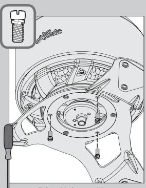
Install three blade assembly screws, found in the X hardware bag.
