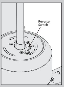
To change the direction of air flow, move the reverse switch to the opposite position.
