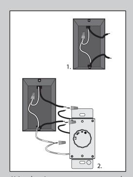
Using the wire connectors, connect each black wire from the wall control to a black wire from the switch box. Connect the green with yellow stripe wire to the grounding wire from the switch box.
