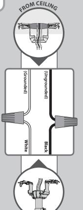
Using the orange wire connectors from the hardware bag, connect the black wire (ungrounded) from the ceiling to the black wire from the fan. Connect the white wire (grounded) from the ceiling to the white wire from the fan.
