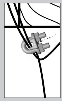
Close the clamp by securely tightening the nuts. Coil up the excess cable.
