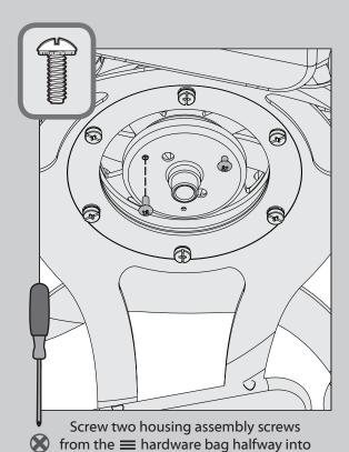
the motor housing. It does not matter
