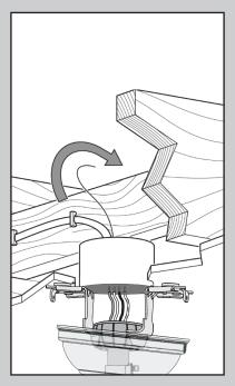
Insert the end of the braided cable through the ceiling bracket and one of the holes in the outlet box into the ceiling. Access the support brace in the ceiling. You may not be able to do this from below the ceiling depending on your installation site.
