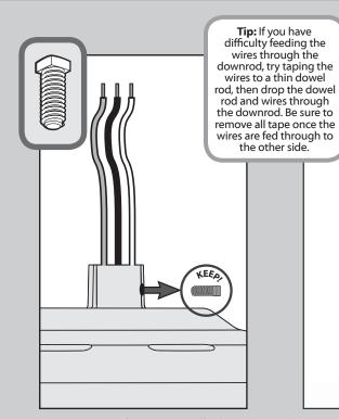
Remove the pre-installed setscrew so that the downrod can be inserted.
