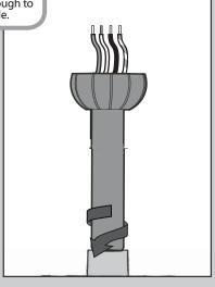
Hand tighten the downrod (at least 4-5 full turns) until it stops.
