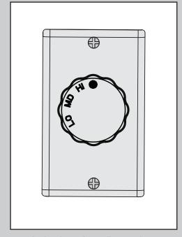
The knob on the wall control unit controls power to the fan. The fan has four speed settings in sequence: high, medium, low and off.
