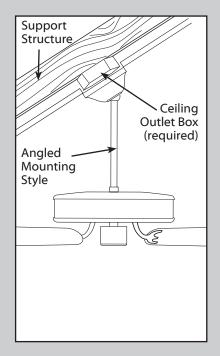
Use **Angled Mounting** to hang the fan from a vaulted or angled ceiling.
