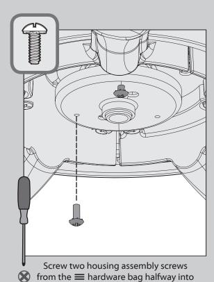
the motor housing. It does not matter
