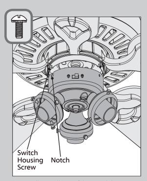
Partially install two of the switch housing screws found in the ≡ bag. Align the notches in the sides of the lower switch housing with the upper switch housing screws. Twist the lower switch housing clockwise to lock into place.
