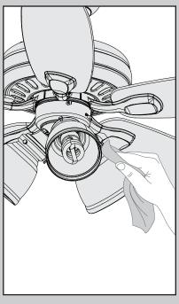
For cleaning the fan, use soft brushes or cloths to prevent scratching. Cleaning products may damage the finishes.
