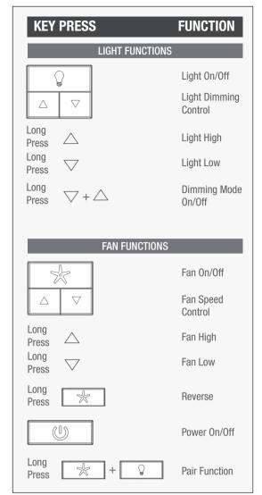
The remote transmitter is already paired to the receiver and ready to use. If you need to pair your remote, cycle power to the fan by turning power off and back on at the wall switch (or circuit breaker if necessary). Within three minutes, do the following:
