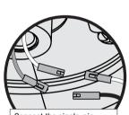
Connect the single-pin connectors from the light kit assembly to the connectors from the fan. Connect the white wires together. Connect the blue and black wires together.
