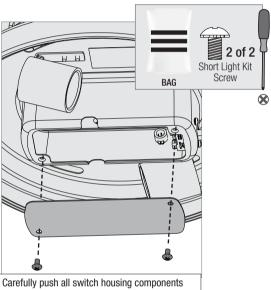
Carefully push all switch housing components into the switch housing, then install the switch housing plate using two short light kit assembly screws, found in the == hardware bag.
