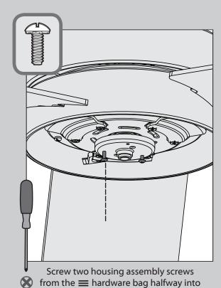
the motor housing. It does not matter
