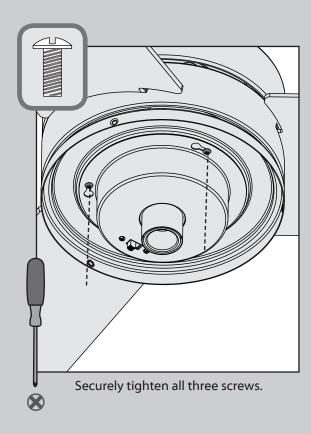
Make sure the lower switch housing is securely attached to the upper switch housing. Failure to properly secure all three assembly screws could result in the light fixture falling.
