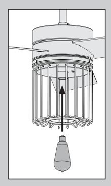
Install a bulb into the socket. When necessary, replace with a bulb of the same type and wattage.
