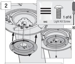
Align the keyhole slots in the top of the light kit assembly with the partially installed assembly screws. Wrap the keyhole slots around the screws and twist counterclockwise. Install the third light kit screw. Tighten all screws securely.
