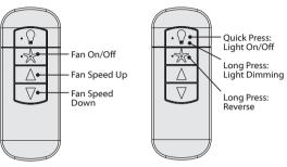
The Fan On/Off button turns the fan on or off. Adjust the fan speed using the "Fan Speed Up" or "Fan Speed Down" directional buttons. Quickly press the Light button to turn the lights off and on. Hold the Light button to raise and dim the light level.
