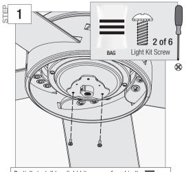
Partially install two light kit screws, found in the hardware bag, halfway into the motor housing as shown. It does not matter which two screw holes you choose.
