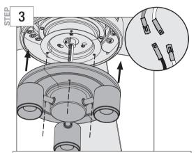
Connect the single-pin connectors from the light kit to the connectors from the fan. Connect the white wires together. Connect the blue and black wires together. Lift the light kit until its screw holes are aligned with the screw holes in the upper switch housing. Make sure all the wires from the light kit are snug inside the center of the light kit, not pinched in between the upper switch housing and the light kit or hanging out of the sides.
