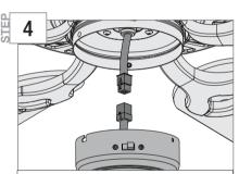
Connect the plugs from the upper and lower switch housings. Make sure to line up the colored markings on the connectors.
