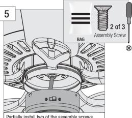
Partially install two of the assembly screws found in the === hardware bag. Align the notches in the sides of the lower switch housing with the screws on the upper switch housing. Twist the lower switch housing clockwise to lock into place.
