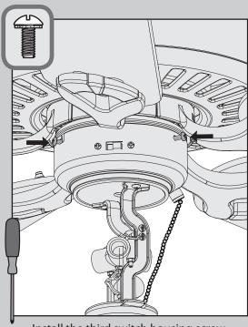
Install the third switch housing screw.
