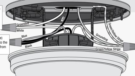
Connect the three grounding wires (green, green/yellow stripe, or bare copper) coming from the ceiling, downrod, and hanging bracket.
