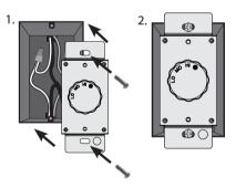
Remove the knob from the wall control and mount the faceplate (not included) to the wall control using the two #6-32 screws you removed earlier from the faceplate.
