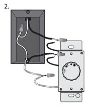
Installing the Wall Control
