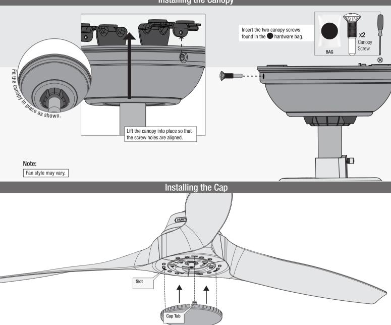
Align the tabs of the cap with the slots of the fan assembly and lift and insert. Cap
