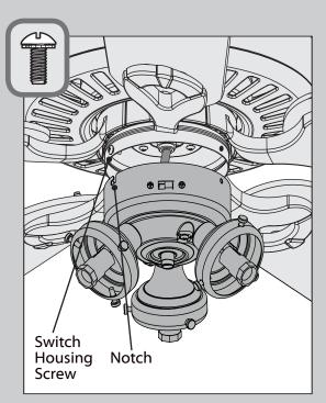
Partially install two of the switch housing screws found in the ≡ bag. Align the notches in the sides of the lower switch housing with the screws on the upper switch housing. Twist the lower switch housing clockwise to lock into place.
