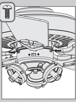
Install the third switch housing screw.
