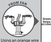
connector from the  $\bigstar$  hardware bag, connect the 3 grounding wires (green, green/ yellow stripe, or bare copper) coming from the ceiling, downrod, and hanging bracket.
