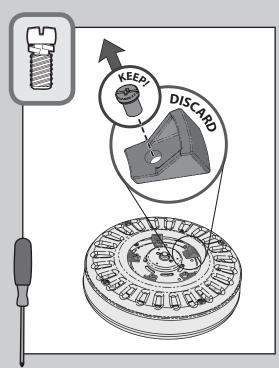
Remove the shipping blocks from the motor. Save the screws. They will be needed for blade iron installation.
