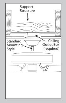
Use **Standard Mounting** or **Low-Profile Mounting** to hang the fan from a flat ceiling.
