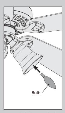
Install a bulb into each of the sockets. When necessary, replace with bulbs of the same type and wattage.
