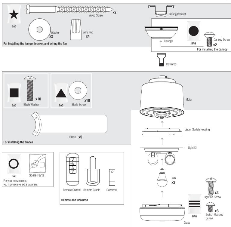
For installing the light kit
