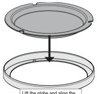
Lift the globe and align the notches in the globe retainer with the tabs in the light kit.
