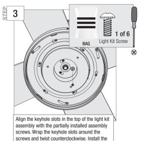
third light kit screw. Tighten all screws securely.
