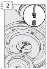
Connect the plugs from the fan and light fixture. Make sure to line up the colored markings on the connectors.
