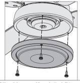
Lift the globe assembly and attach it to the upper switch housing using the three thumbscrews, found in the == hardware bag. Tighten all three screws securely by hand.
