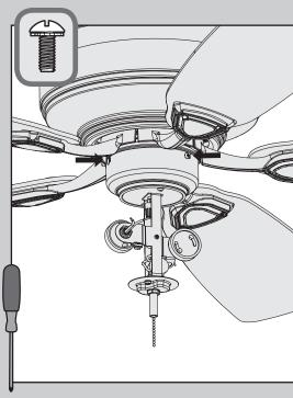
Install the third switch housing screw.
