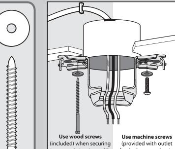
(included) when securing to support structure with approved electrical outlet box. Drill 9/64" pilot holes in support structure to aid in securing ceiling bracket with hardware found in the ★ hardware bag.
