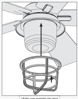
Lift the cage assembly into place
