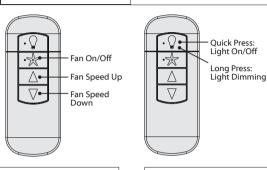
The Fan On/Off button turns the fan on or off. Adjust the fan speed using the "Fan Speed Up" or "Fan Speed Down" directional buttons.
