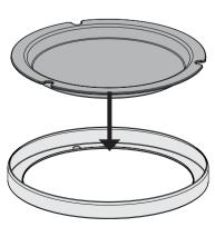
Lift the globe and align the notches in the globe retainer with the tabs in the light kit.
