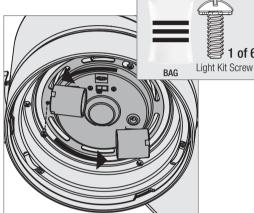
Turn the light kit counterclockwise until the light kit screws are firmly situated in the narrow end of the keyhole slots. Install the third screw and tighten all three screws securely.
