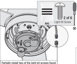
Partially install two of the light kit screws found in the = bag. It does not matter which two screw holes you choose. Connect the plugs from the upper and lower switch housings. Make sure to line up the colored markings on the connectors.
