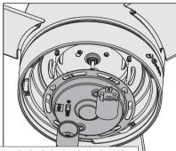
Align the keyhole slots in the light kit housing with the two screws. Make sure all the wires from the fan and the light kit are snug inside the center of the light kit, not pinched in between the upper switch housing and the light kit or hanging out of the sides.
