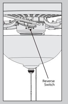
**Changing the direction of air flow** - move the reverse switch to the opposite position.
