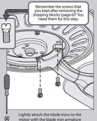
motor with the blade iron armature screws, then securely tighten after both screws are attached.
