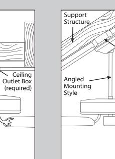
Use Standard Mounting or Low-Profile Mounting to hang the fan from a flat ceiling.
