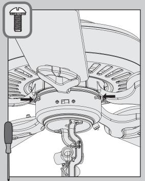
Install the third switch housing screw. Tighten all three screws securely.
