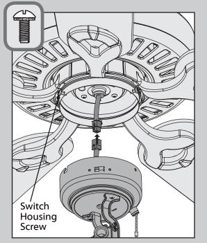
Partially install two of the switch housing screws found in the ≡ bag. Connect the plugs from the upper and lower switch housings. Make sure to line up the colored markings on the connectors.
