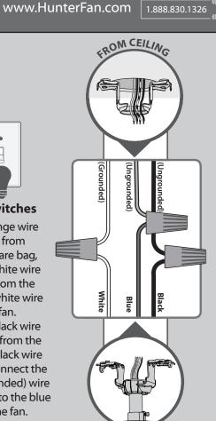
Turn the splices upward and push them carefully back through the hanger bracket into the outlet box. Spread the wires apart, with the grounded wires on one side of the outlet box and the ungrounded wires on the other side of the outlet box.
