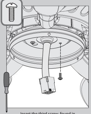
Insert the third screw, found in the ≡ hardware bag, into place and then tighten all three screws.
