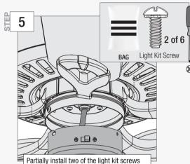
found in the **=** hardware bag. Align the notches in the sides of the lower switch housing with the screws on the upper switch housing. Twist the lower switch housing clockwise to lock into place.
