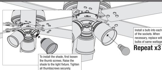
of the sockets. When necessary, replace with bulbs of same wattage
