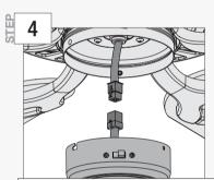
Connect the plugs from the upper and lower switch housings. Make sure to line up the colored markings on the connectors.
