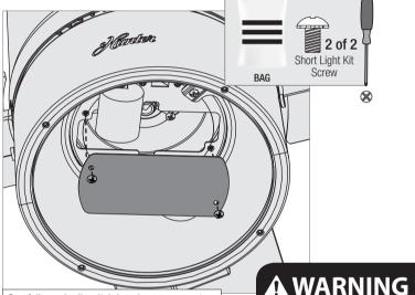
Carefully push all switch housing components into the switch housing, then install the switch housing plate using two short light kit assembly screws, found in the hardware bag.
