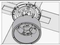
Align the keyhole slots in the top of the light kit assembly with the partially installed assembly screws. Wrap the keyhole slots around the screws and twist counterclockwise.
