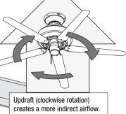
creates a more indirect airflow. Updraft airflow is great for moving warm air downward.
