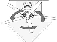
Ceiling fans work in two directions: downdraft (counterclockwise rotation) and updraft (clockwise rotation). To change the direction of air flow, turn the fan off and let it come to a complete stop. Slide the reversing switch to the opposite position. Restart the fan.
