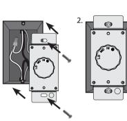
5 Installing the Wall Plate Remove the knob from the wall control and mount the faceplate (not included) to the wall control using the two #6-32 screws you removed earlier from the faceplate.
