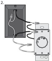
4 Installing the Wall Control Insert the wall control into the outlet box and secure the two metal tabs to the tabs on the switch box using the two flat head screws that came with the switch box.
