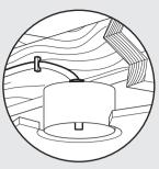
You must be able to secure the fan to building structure or fan-rated outlet box.
