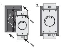
Remove the knob from the wall control and mount the faceplate (not included) to the wall control using the two #6-32 screws you removed earlier from the faceplate.
