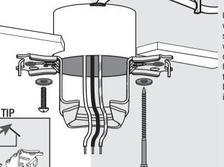
Use wood screws and washers (included) when securing to support structure with approved electrical outlet box. Drill 9/64" pilot holes in support structure to aid in securing ceiling bracket with hardware found in the  $\bigstar$  hardware bag.
